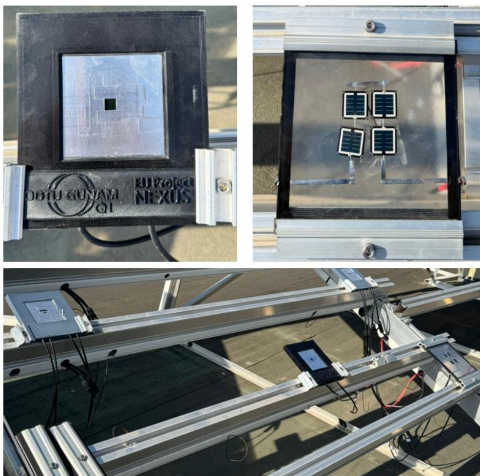
Figure 5. O1 and 4-cell minimodules at the outdoor test station (Ankara, Türkiye)
