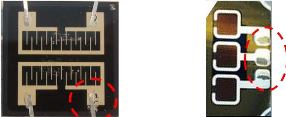
Figure 2: Examples of contact failure occurring both with the metallization and the top cell layer are ripped off.
